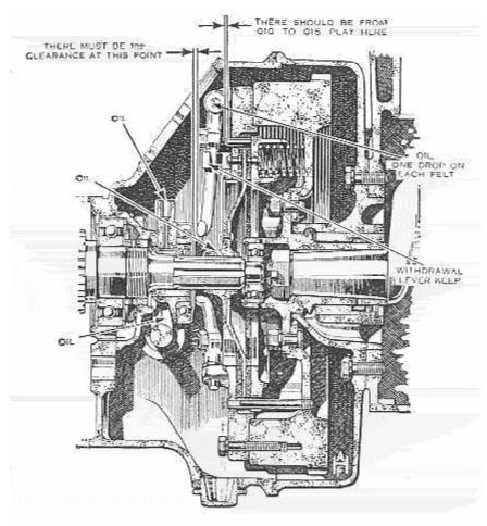
All right, all right! Sit down there at the back, ladies and gentlemen! The clutch is a simple mechanism which, given a fair chance, will function efficiently without even a lot of maintenance. Unfortunately many owners are inclined to leave it too much to its own devices. In the end the devices become worn and finally pass out - in small pieces of metal and metal dust - through holes which they make for themselves in the bell-housing!
