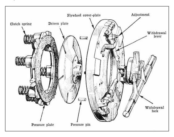
For those interested in strengthening the clutch, fitting the larger MG J2 clutch is well worth considering. The existing Minor flywheel can be easily modified to take a J2 driven and pressure plate by simply repositioning the guide pins. Take (plenty of) metal out from inside the rim, and move the guide pins out. The J2 has shorter pins on a step inside the flywheel. Therefore, don't use J2 guide pins, as you can remove more metal by retaining the original long-type Minor pins.
